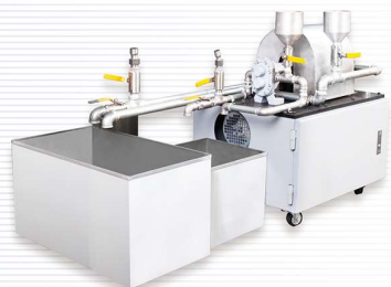
涂料供给装置 Coating supply device
